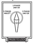
Figure 22. Voltage Selector Switch 240/139V
