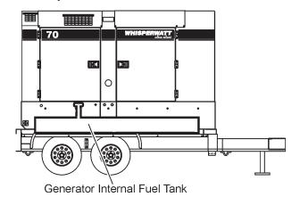
Figure 32. Internal Fuel Tank System
