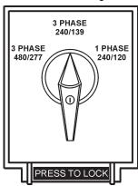
Figure 16. Voltage Selector Switch
