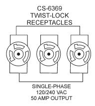
Figure 10. 120/240V Twist-Lock Auxiliary Receptacles
