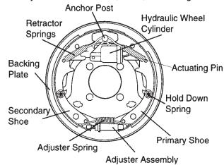
Figure 57. Hydraulic Brake Components
