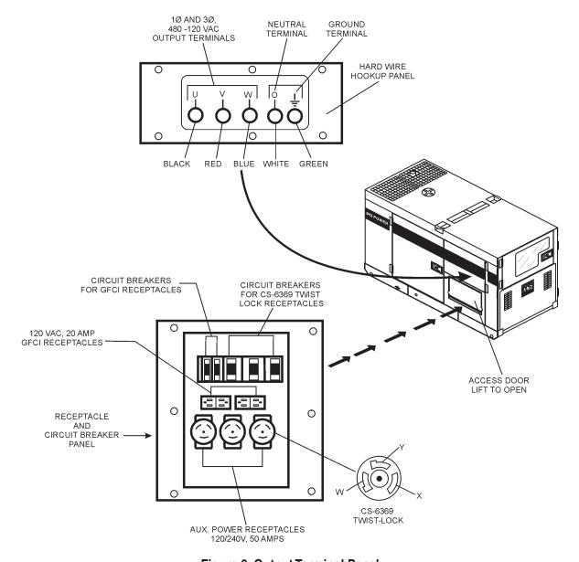
Figure 8. Output Terminal Panel
