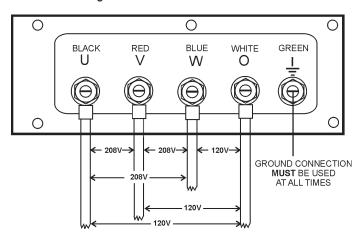
Figure 26. Output Terminal Lugs 3Ø-208V/120V Connections
