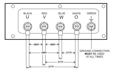
Figure 28. UVWO Terminal Lugs 480/277V Three Phase Connections
