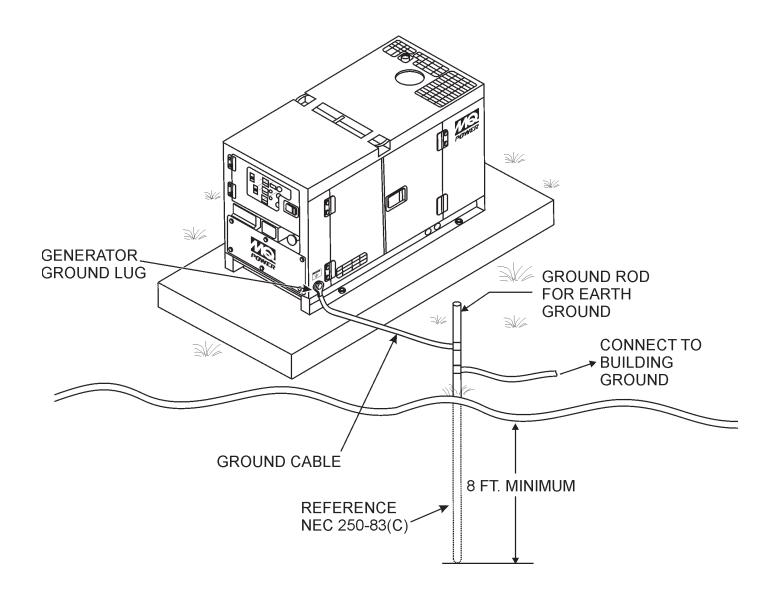
**Figure 4. Typical Generator Grounding Application**
