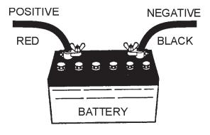
Figure 38. Battery Connections
