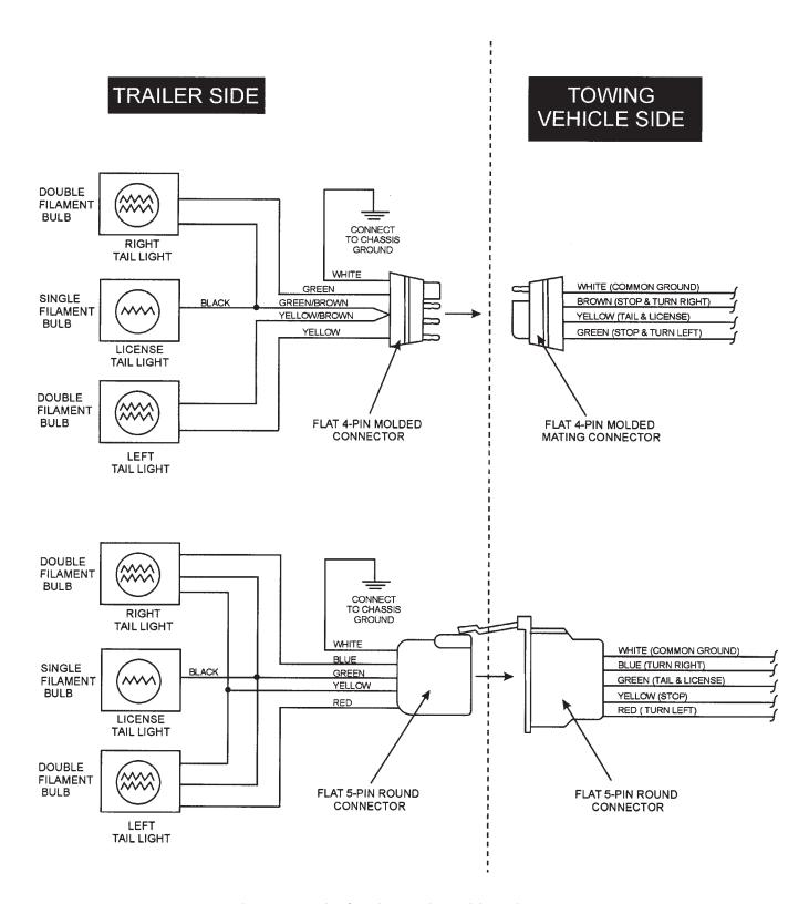
Figure 60. Trailer/Towing Vehicle Wiring Diagram
