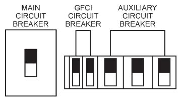
Figure 52. Main, Aux. and GFCI Circuit Breakers (ON)
