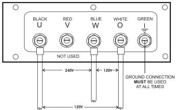
Figure 30. UVWO Terminal Lugs 1Ø-240V/120V Connections
