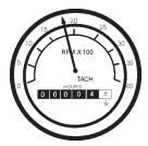
Figure 51. Engine Tachometer Gauge
