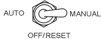
**Figure 50. Auto-Off/Reset-Manual Switch**
