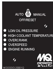
Figure 11. Engine Controller
