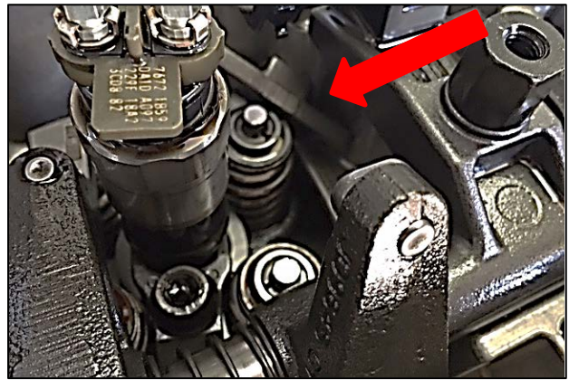
Valve bridge dropped
