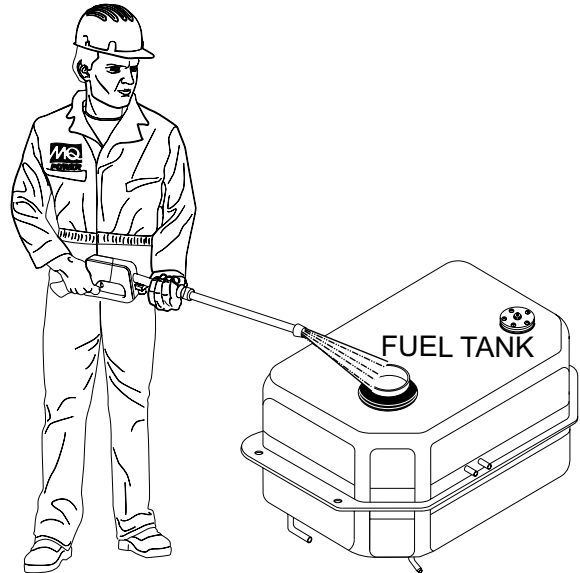
Figure 60. Fuel Tank Cleaning
