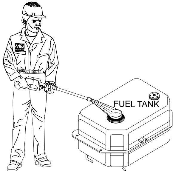
Figure 60. Fuel Tank Cleaning
