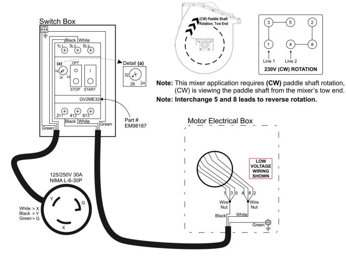
BALDOR RELIANCE SPEC: 37E365W796 VOLT: 230, PH: 1, HZ: 60, HP: 5, AMPS: 22, RPM: 1725
