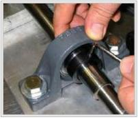
Photo shows collar installed on mixer paddle shaft.
