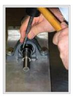
**4.** After collar has engaged, tighten set screw to ensure the collar does not move.
