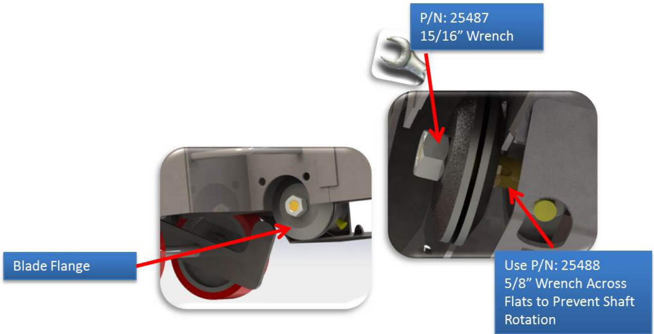
Figure 5. Blade Flange Removal
