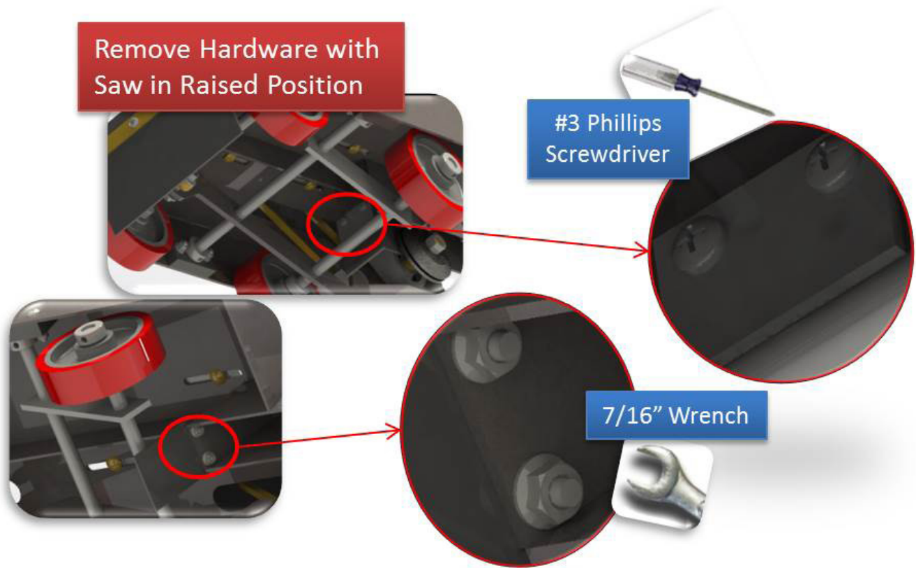
Figure 3. Slurry Guard and Mount Plate Removal
