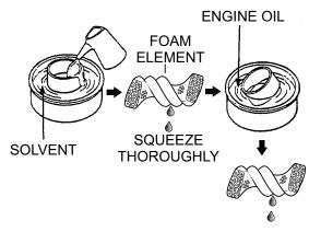
Figure 31. Cleaning Foam Element
