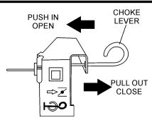
Figure 14. Choke Lever
