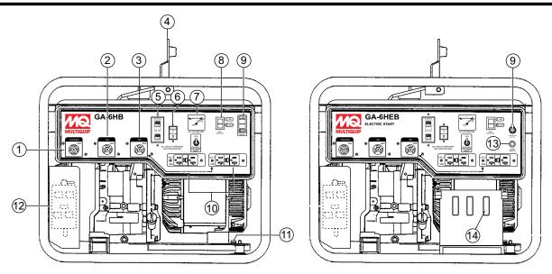
**Figure 3. Generator Components**
