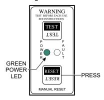
Figure 40. GFCI Module (Green LED ON Reset)
