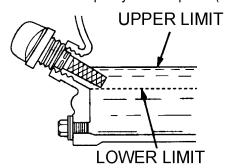
Figure 10. Engine Oil Dipstick(Oil Level)
