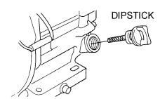
Figure 9. Engine Oil Dipstick Removal
