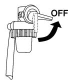
Figure 26. Engine Fuel Valve Lever (OFF)
