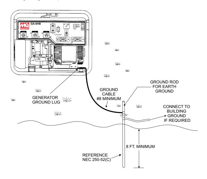
Figure 2. Generator Grounding
