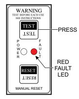
Figure 37. GFCI Module (Red/Fault LED ON)
