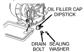
Figure 29. Draining Engine Oil
