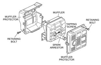
Figure 32. Spark Arrester Removal
