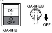
Figure 18. Idle Control Switch (OFF)
