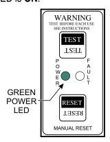
Figure 36. GFCI Module (Green LED ON)
