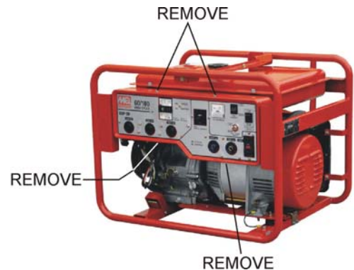
Figure 1. GDP-5H Control Panel Removal
