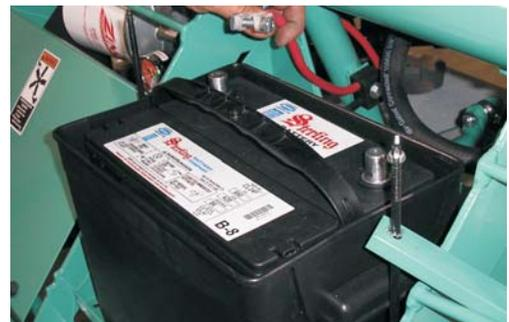
Figure 3. Disconnect Battery Cables
