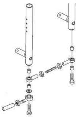
This is the assembly arrangement of current production with the new rod ends, spacer and coupling nut. Notice the location of the linkage
