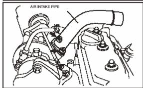
**Step 6**: Remove the Rocker Cover by removing the 3 nuts on the top of the cover. Carefully remove the breather hose from the Rocker Cover.
