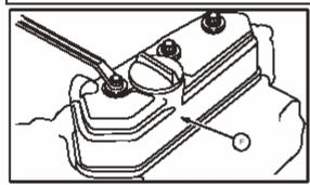
**Step 7**: Ensure the new Rocker Cover Gasket is properly seated in the new Rocker Cover. Install the new Rocker Cover using the nuts and washers from the original cover. **Torque nuts to 50 in. lbs.**
