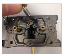
Using Cabinet screwdriver, remove pilot and main jets noting position for proper reinstallation. Thoroughly clean both pilot jets.
