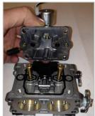
Remove all O-rings and gaskets before spraying (cleaning) carburetor body.
