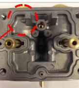
Arrow represents direction of input when reassembling the float pin. —
