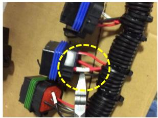
4. Use a butt connector to connect the black wire from the service kit to the black wire on the wire harness and heat shrink for insulation.
