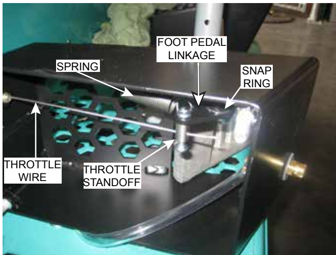
Figure 18. Throttle Wire Removal
