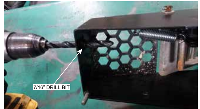
Figure 20. 7/16" Expanded Drill Lock Nut
