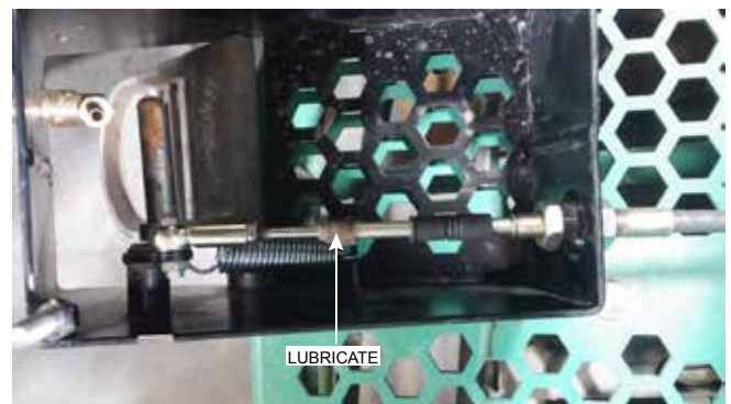
Figure 21. Foot Pedal Cable Assembly
