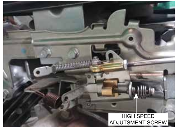
Figure 24. High Speed Adjustment Screw
