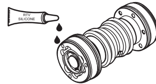
Figure 27. Applying RTV Silicone
