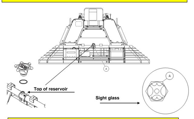
WITH THE MACHINE COLD AND NOT RUNNING, CAUTION! Only run the engine long enough to check the oil level. Start the unit and throttle the engine ½ to ¾ speed, check oil level as described in step one, add oil if needed, install oil fill cap and shut engine off.
