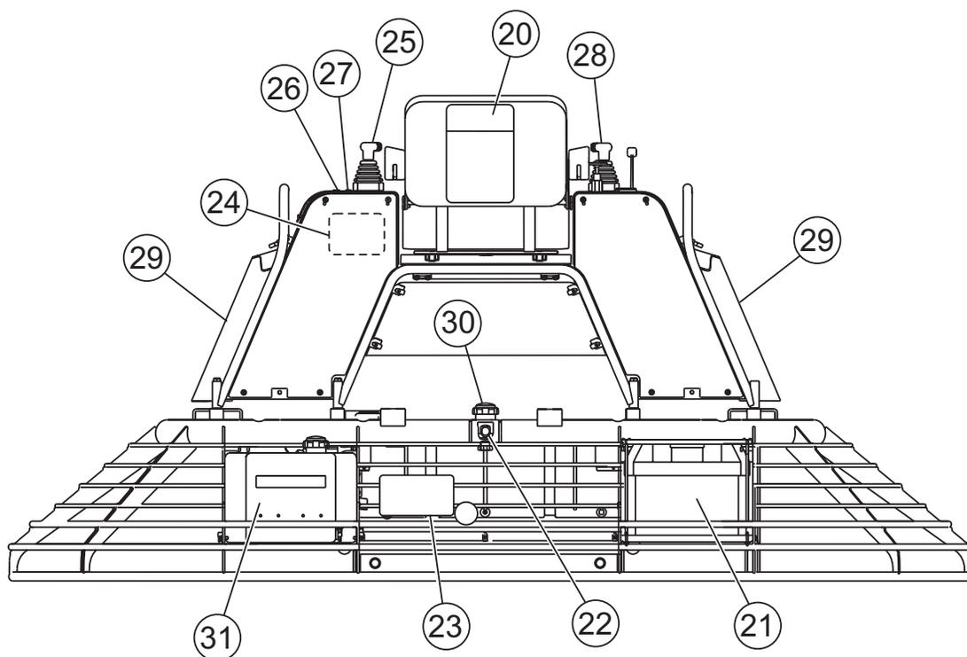
**Figura 4. Controles y componentes HTX-YANMAR DIESEL (vista trasera)**
