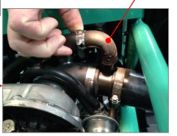
• Loosen clamps, remove and replace joint breather.
