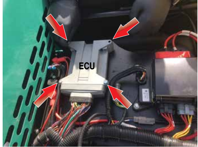
Figure 12. ECU Bolt Removal
