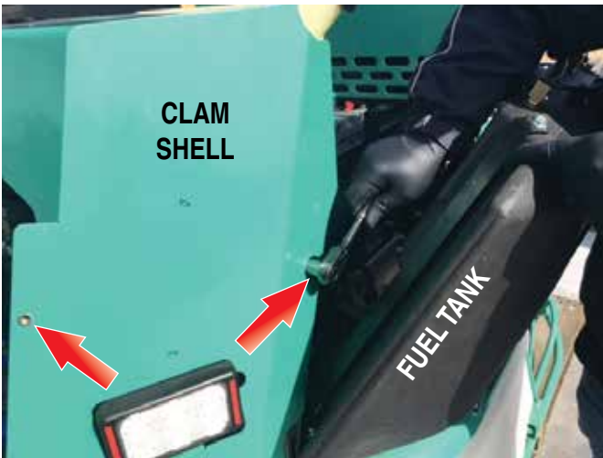
Figure 10. Clam Shell Bolt Removal
