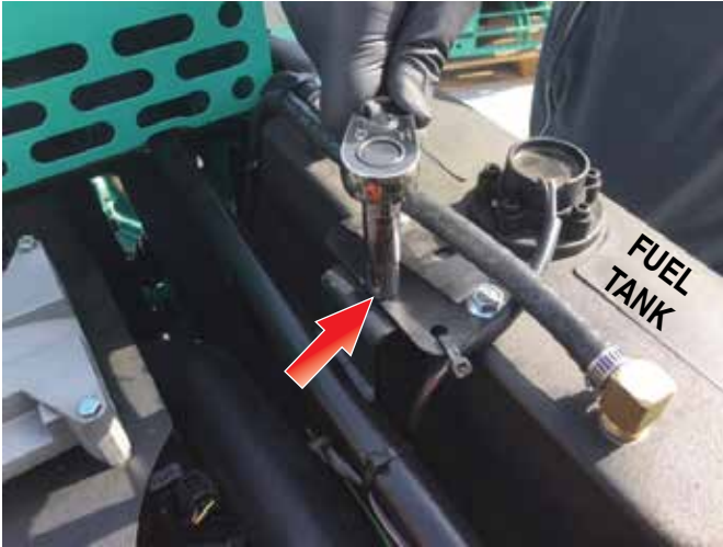
Figure 9. Fuel Tank Bolt Removal
