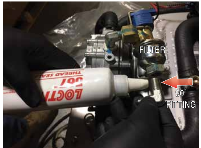
Figure 17. Applying Loctite® 567™ (90° Fitting)
