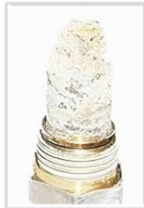
Excessive DEF Buildup on NOx Sensor
