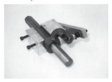
Shown here is the adjustment fixture with an arm. As each arm is locked into the fixture, the arm bolt is adjusted to where it contacts a stop on the fixture. This will consistently adjust all of the trowel arms, keeping the finisher as flat and evenly pitched as possible. See Blade Pitch Adjustment Procedure in the Maintenance section of this manual for more information.
