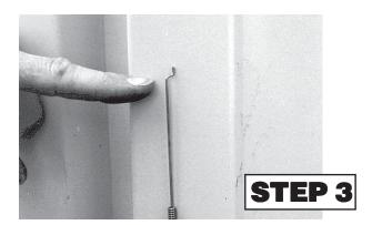
On Robin engines, the hook on the engine end of the throttle wire must be removed. Make the cut as shown (Step 3). The rest of the engine will not require this modification to the throttle cable.
