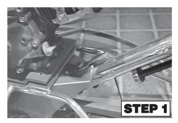
second bolt carries the auxiliary lift handle bracket in the place of a washer.
