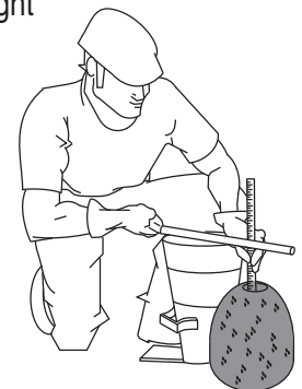
Figure 54-F. Slump Test (Measurement)
