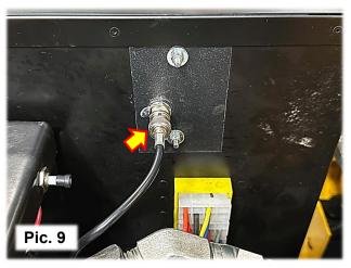
10. Using plastic tie straps, secure the coaxial cable as needed to the large electrical loom going up to the back of the control box.
