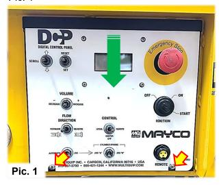
2. Carefully lower the front control panel, flip it over and securely place it as shown in Pic. 2-A to expose the control box interior and still be able to reach behind the control box. (Use care not to pull wires from the key switch).
