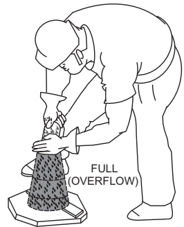
Figure 69-C. Slump Test (Full-Overflow)
