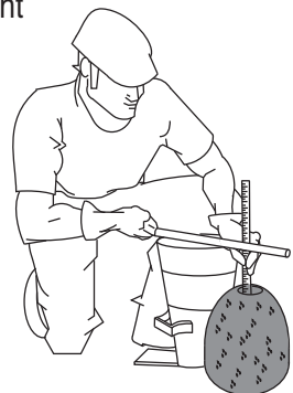
Figure 69-F. Slump Test (Measurement)
