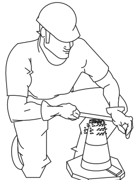
Figure 69-D. Slump Test (Removing Excess Concrete)
