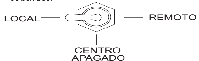
Figura 26. Interruptor de control de bombeo (LOCAL)
