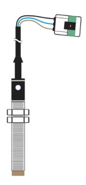
Note: Using a test light with an incandescent type bulb will overload the sensor's output ground circuit if its amp rating is unknown and over this circuit's capacity of 250 mA. This would cause the sensor's overload protection to engage causing the sensor's function display switching status L.E.D. to be disabled.
