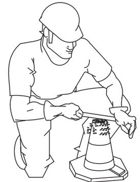
Figure 68-D. Slump Test (Removing Excess Concrete)
