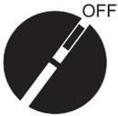
**ALWAYS** place the **Engine ON/OFF** switch in the **OFF** position. **NEVER** perform maintenance on the unit with the ignition key in the **ON** position.
