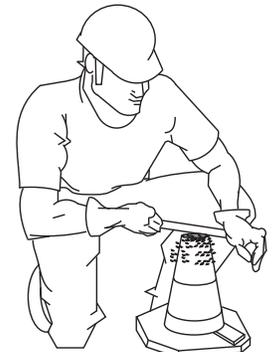
Figure 68-D. Slump Test (Removing Excess Concrete)
