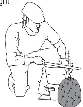
Figure 68-F. Slump Test (Measurement)
