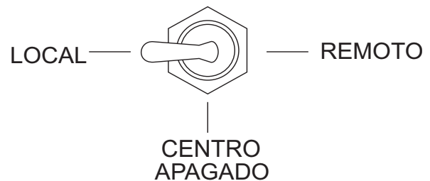
Figura 26. Interruptor de control de bombeo (LOCAL)
