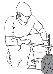
Figure S. Slump Test (Measurement)
