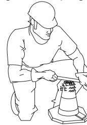
Figure Q. Slump Test (Removing Excess Concrete)
