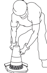
Figure R. Slump Test (Cone Invert)
