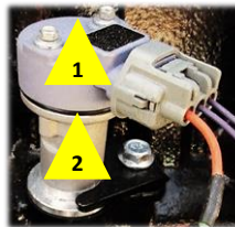
(1) Cam Position Sensor P/N 200344 (2) Cam Synch. P/N 201338
