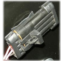
Comm. Conn. (Data Link) "Diagnostic Software Kit P/N 202163"
