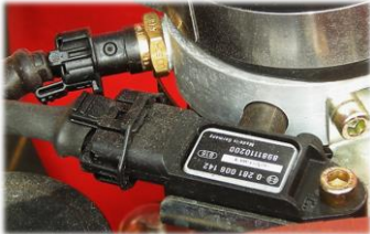
Air filter down pressure sensor (AFDPS) & Air temp sensor (ATS)
