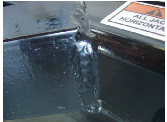
Figure 4. Triple Pass Weld
