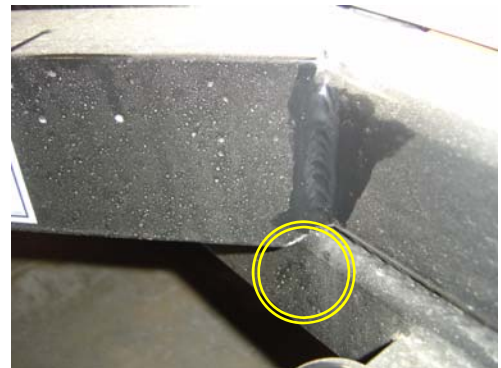
Figure 3. Single Pass Weld
