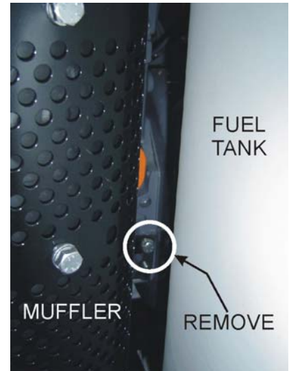
Figure 7. Muffler Bracket Removal
