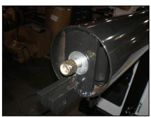
Install pulley and pin clevis onto swivel base and secure with cotter pin
