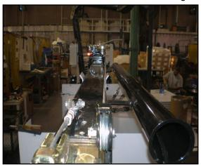
Tap all six T-bar cover plate holes using a 10/32 tap. Install cord grip. Install twelve inch long (14 gauge) ground strap. Install four female wire receptacles as shown below.
