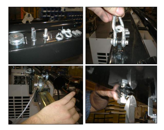
Run upper mast cable through pulley and shackle, secure cable with two swage clamps
