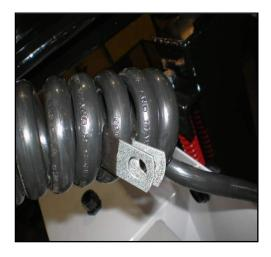
Wrap cable around mast as seen in picture one time. Pull cable slack through clamp located in front panel until cable pulls tight to swivel base mounting bolt as seen below.
