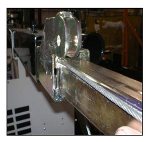
Insert four mast slide blocks in between lower mast and mast housing and secure with rivets, repeat steps for upper mast between and lower mast. Be sure to keep cables aligned with pulley brackets, see below.
