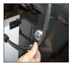
Using trailer mounted winch, raise mast where support pin is not protruding into mast housing. Install winch on mast tube seen below.
