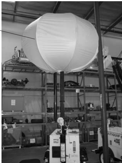
Figure 16. Installed Balloon with Mast Raised
