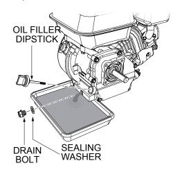
Figure 28. Draining Engine Oil
