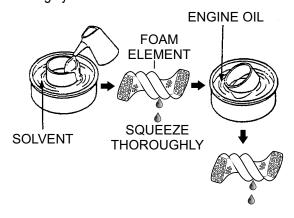
Figure 30. Cleaning Foam Element
