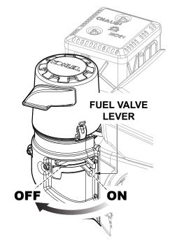
Figure 25. Fuel Shut-Off Lever (OFF)
