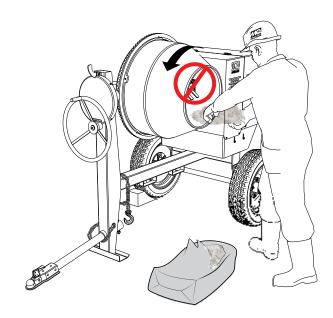
Figure 22. Filling Mixing Drum (WRONG)
