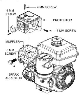
Figure 31. Spark Arrester
