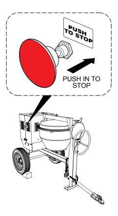
Figure 24. Start/Stop Button (Stop Position)
