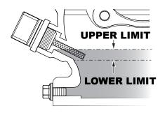
Figure 10. Engine Oil Dipstick (Oil Level)
