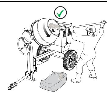
Figure 21. Filling Mixing Drum (CORRECT)
