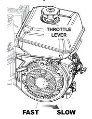
Figure 23. Throttle Lever (Idle)
