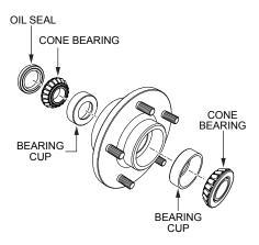
Figure 35. Wheel Hub and Bearings
