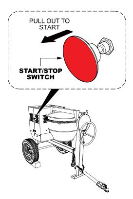
Figure 18. Engine Start/Stop Button
