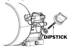
Figure 9. Engine Oil Dipstick (Removal)
