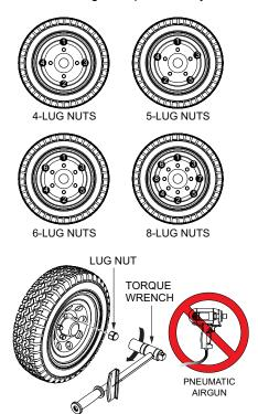
Figure 38. Wheel Lug Nuts Tightening Sequence
