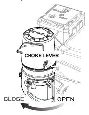
Figure 15. Choke Lever
