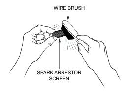
Figure 32. Cleaning The Spark Arrester
