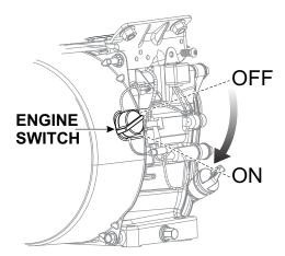
Figure 17. Engine On/Off Switch
