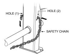
Figure 6. Attaching Safety Chains to Mixer Stand
