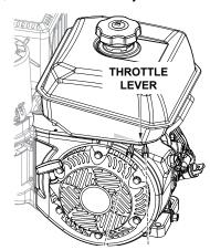
Figure 16. Throttle Lever
