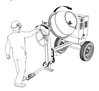
Figure 20. Mixing Drum Positioning
