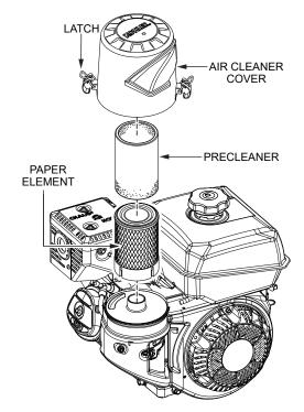
Figure 29. Engine Air Cleaner (Quad-Clean)
