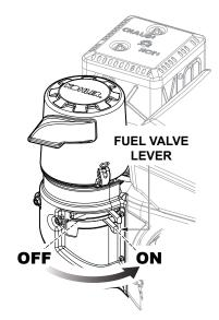
Figure 14. Fuel Shut-Off Lever
