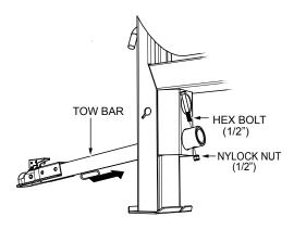
Figure 5. Inserting Tow Bar
