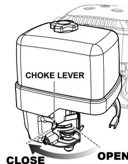
Figure 24. Choke Lever
