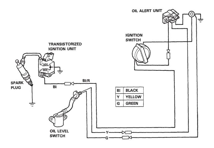
Figure 37. Honda GX270 QWH2 Engine Wiring Diagram
