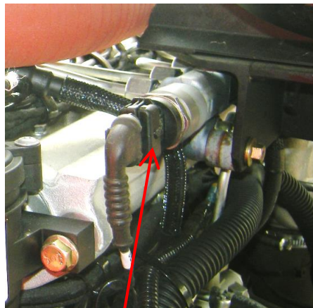
Rail Pressure Sensor (RPS) / (RDS) wire Max pressure 1,800 bar (26,100 PSI)
