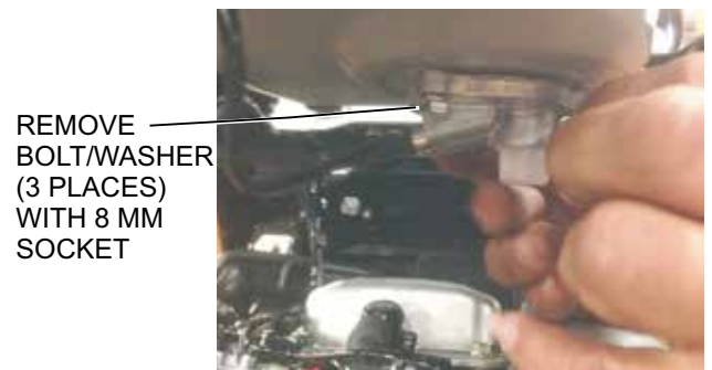
Figure 18. Filter Holder Removal
