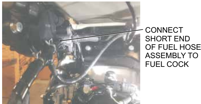
Figure 24. Fuel Hose (Short) Connection
