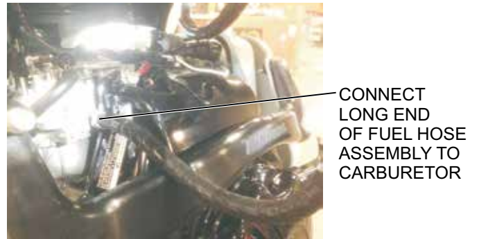
Figure 25. Fuel Hose (Long) Connection
