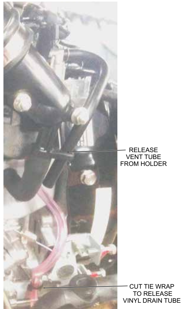
Figure 5. Releasing Vent and Drain Tubes
