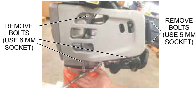
Figure 2. Cover Removal
