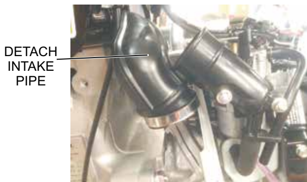
Figure 4. Detaching Intake Pipe
