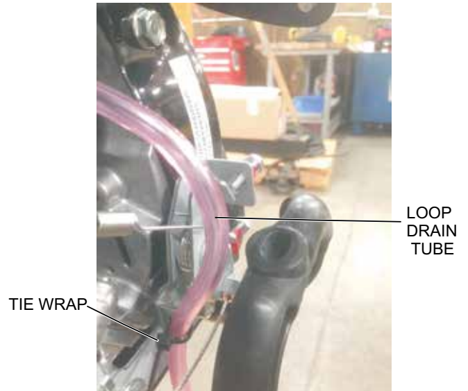
Figure 17. Securing Drain Tube
