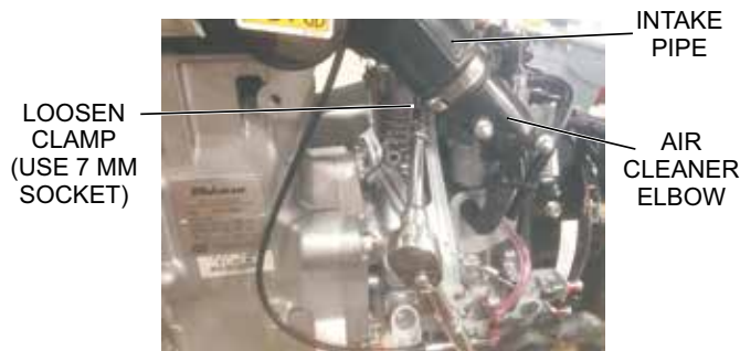
Figure 3. Loosening Intake Pipe Clamp
