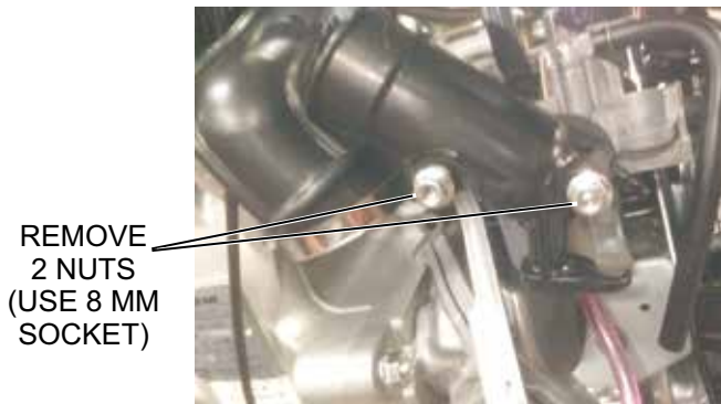
Figure 7. Air Cleaner Elbow Removal
