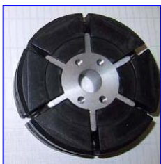
Old Clutch Mounting Tool MQ part # (9830-10060)
