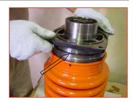
Expanding the bellows during assembly makes it easier to insert the cylinder guide.
