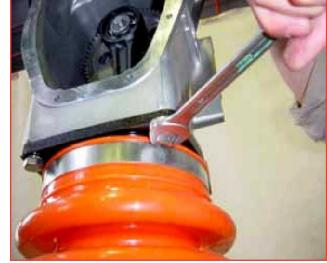
With the (4) mounting bolts removed, raise the top assembly to access and remove the piston pin.
