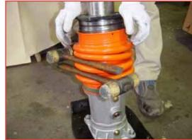
After inserting aluminum lock pin and assembling clamps ensure the clamps are within the designated grooves on the bellows.
