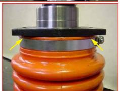
After re-joining the connecting rod to the bottom end, apply Loctite # 221 (red high strength) to the crankcase mounting bolts and torque to spec.
