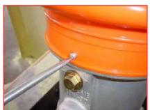
After removing bottom lock pin, remove bellows from oil reservoir.
