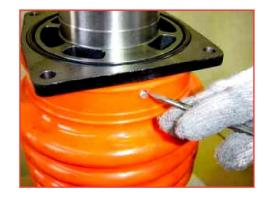
After removing top lock pin, remove the cylinder guide. It may be necessary to use pry-bars.
