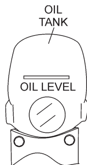
Figure 7. Oil Tank (Front View)
