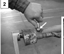
2- Remove the 3 screws that secure the Pitch Control Housing to the Tower Tube end.
