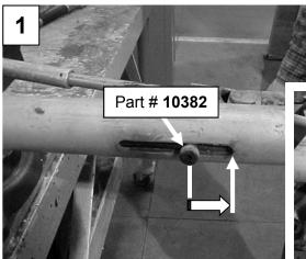
1- By cranking the Handle counter clockwise, position the Shoulder Bolt part # 10382 to the top end of the slotted hole.
