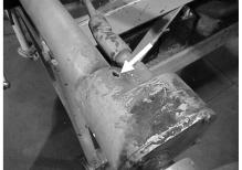
3- While securely supporting the Pitch Control Housing by hand, crank the Handle clockwise until the Pitch Control Housing separates completely from the Tower Tube.
