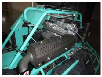
Figure 11. New Muffler Installed 15. Reconnect the battery cables on the machine.
