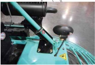
Figure 9. Muffler Vibration Clamp Installation
