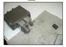
Insert the big ball (part. 7.3) into the hole of the spindle next to the small balls. (part. 7.4)
