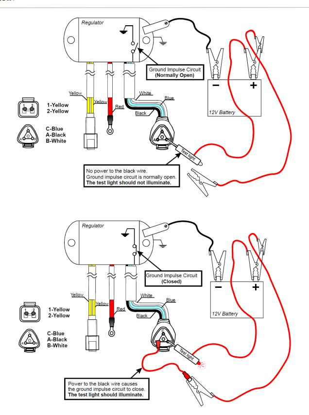
**NOTE**: If regulator is found to be defective. Before replacing it ensure alternator is functioning properly - inspect alternator wires for short to ground.
