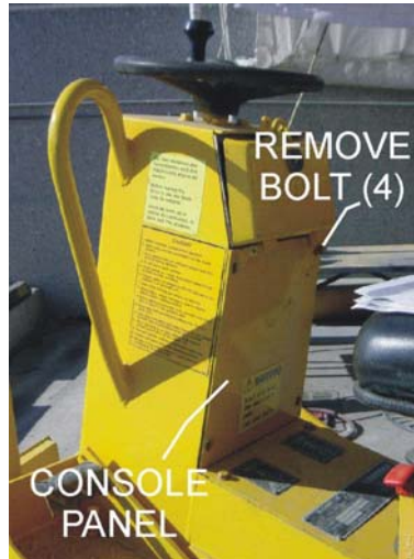
Figure 4. Console Panel Removal
